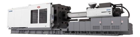
The installed Nissei 950-ton press is equipped with Yushin Automation and features a 600L injection unit with a 112 mm screw and a 210-ounce shot capacity, designed to support customers in the power backup and other key industries. This brings the total number of presses at the Newton Falls plant to 19, with capacities ranging from 55 to 1,440 tons.
