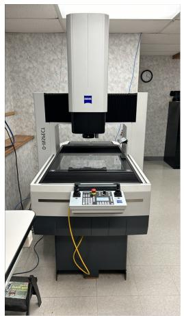
To further enhance quality control, the Zeiss O-Inspect 543 was added, combining tactile probing precision with advanced optical measurement technology. This cutting-edge equipment offers several key features:
